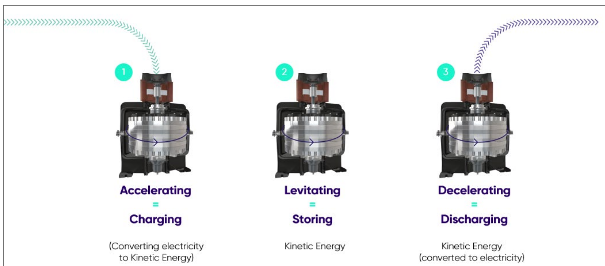
Diagram 1. The operating modes of a flywheel
