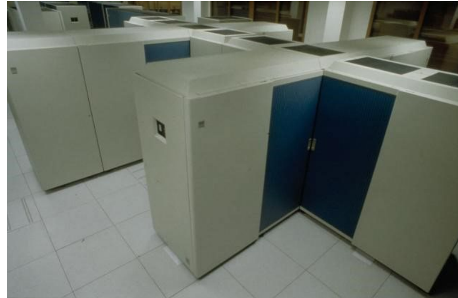
DLC - IBM 3090-400 1988 - Cold Plate
