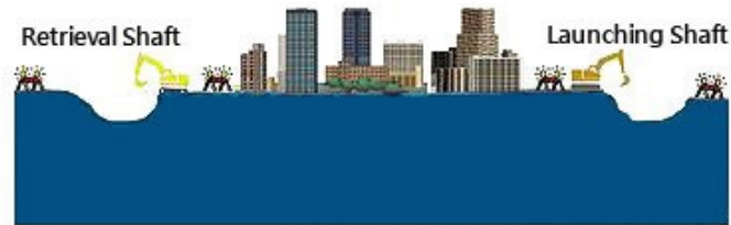
1. Excavate launching shaft and retrieval shaft
