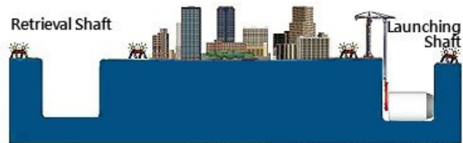
2. Assemble the TBM at the launching shaft
